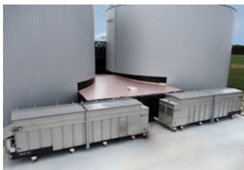
2 solid dosing systems type BIG-Mix 118 m³ with a total capacity of 236 m³
