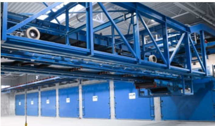
Tunnel filling hall, fermenter and tunnel filling unit (Poznań/PL)
